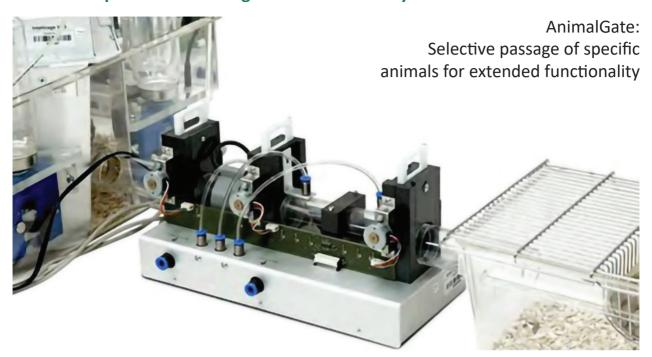
Senses the direction of movement & allows/denies passage to satellite cage
