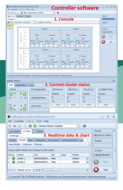
Experimental files from the Designer are loaded and executed by the Controller software
